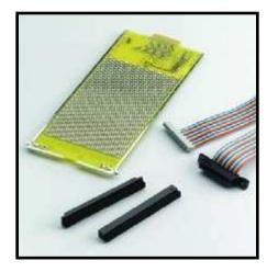
The Model 7061 was designed with a 6-volt supply, ground trace, and a grid pattern of platedthrough holes on 0.1 inch centers for mounting special relays or circuits. Relay drive lines from the scanner mainframe can be used for control. A supplied ribbon cable assembly extends the relay drive lines beyond the enclosure for easy access to relay cards for troubleshooting.
